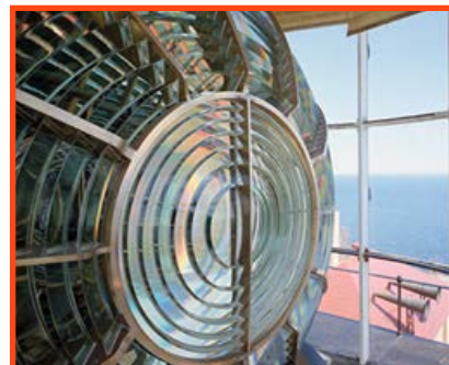
Interior view of Fresnel lens in lantern of Split Rock Lighthouse, Lake County, MN. Jet Lowe, 1990. Prints and Photographs Division, Library of Congress.
