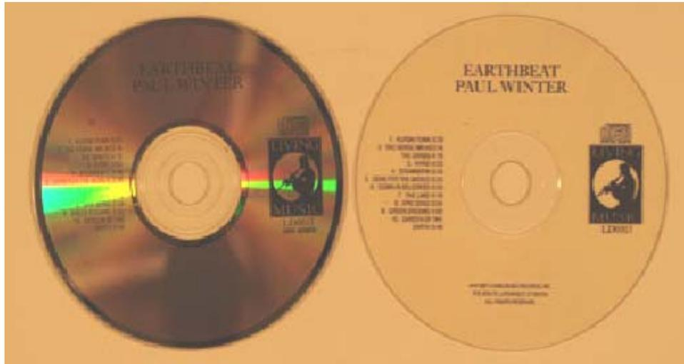
**Image 4. Two CDs after 500 Hours of accelerated aging**
