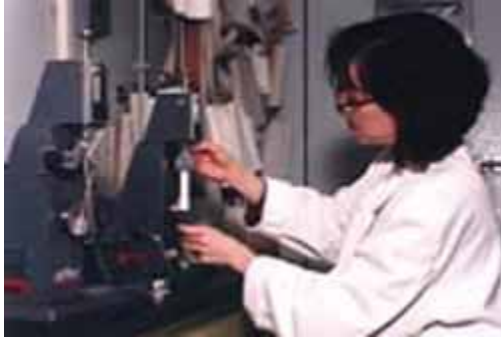
At left: Performing MIT fold endurance test on a paper sample
